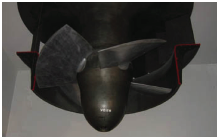
Figure 36 The Kaplan Turbine (Source: Way2Science)
